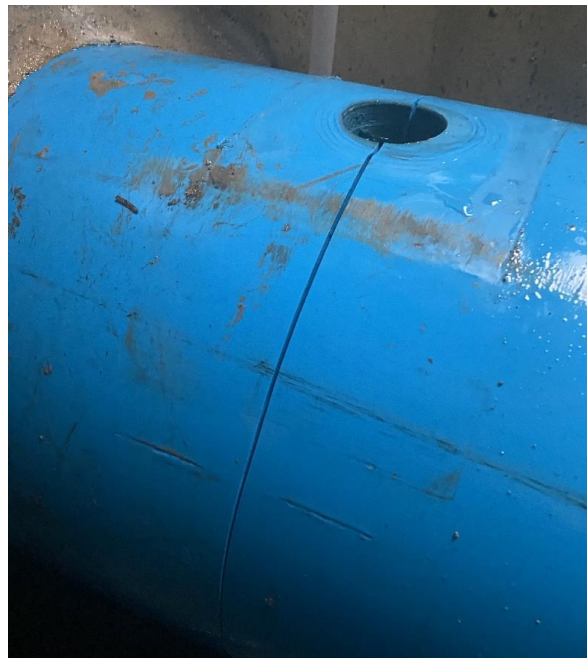
Broken Water Main at Fort Rupert Reservoir
