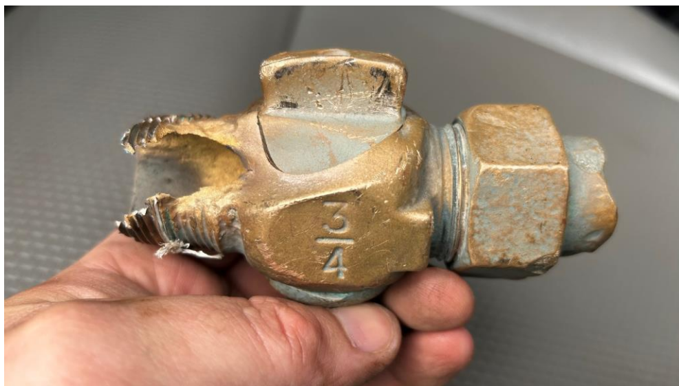
Broken corporation stop found on Steel Road. Estimated leaking at
